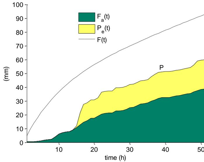
**Figure 3: Infiltration components for Horton's method**
