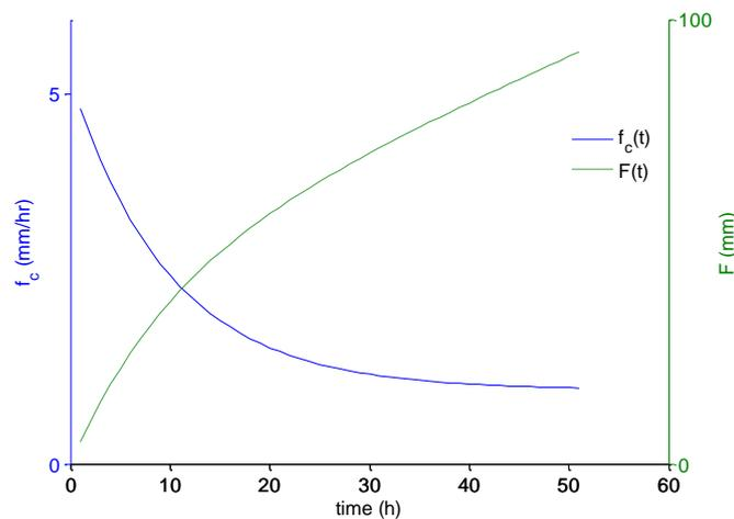
**Figure 1: Infiltration capacity and cumulative infiltration**
