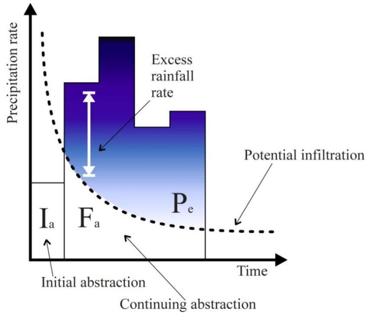
**Figure 4: Infiltration components described by the SCS method**
